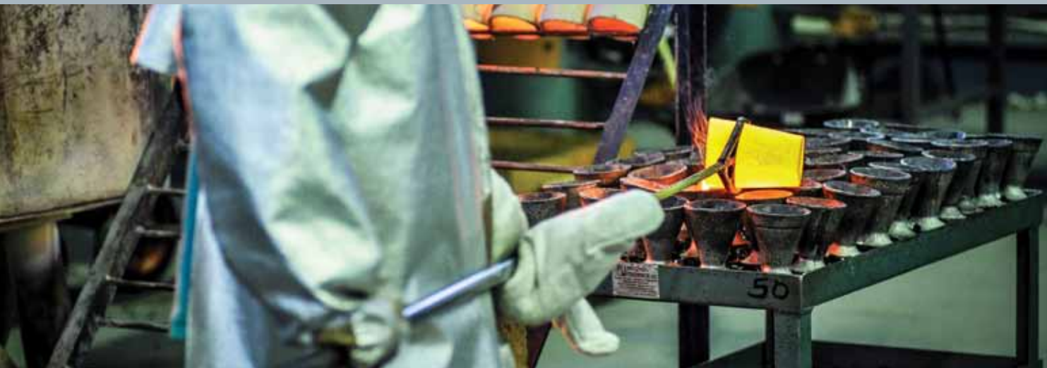
The pouring of molten PGMs during the assay process.
